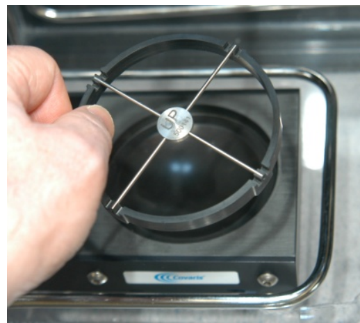
The 500141 Intensifier (left) shown installed in the E-Series transducer well and (right) removed.
