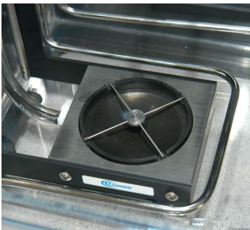
The 500141 Intensifier (left) shown installed in the E-Series transducer well and (right) removed.
