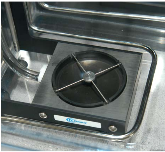
The 500141 Intensifier (left) shown installed in the E System transducer well and (right) removed. Note the “UP” marking at the center of the Intensifier.
