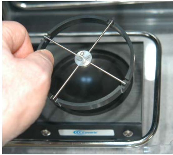
The 500141 Intensifier (left) shown installed in the E System transducer well and (right) removed. Note the “UP” marking at the center of the Intensifier.
